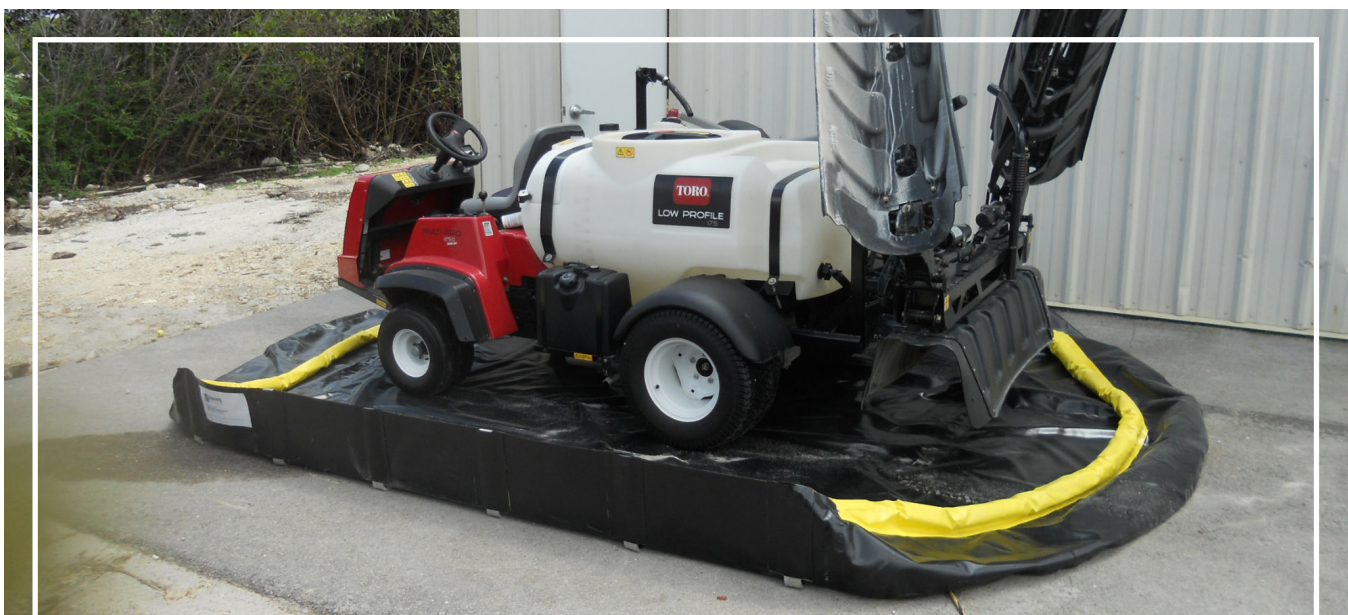
Portable low cost containment systems can provide an effective way to provide containment.
