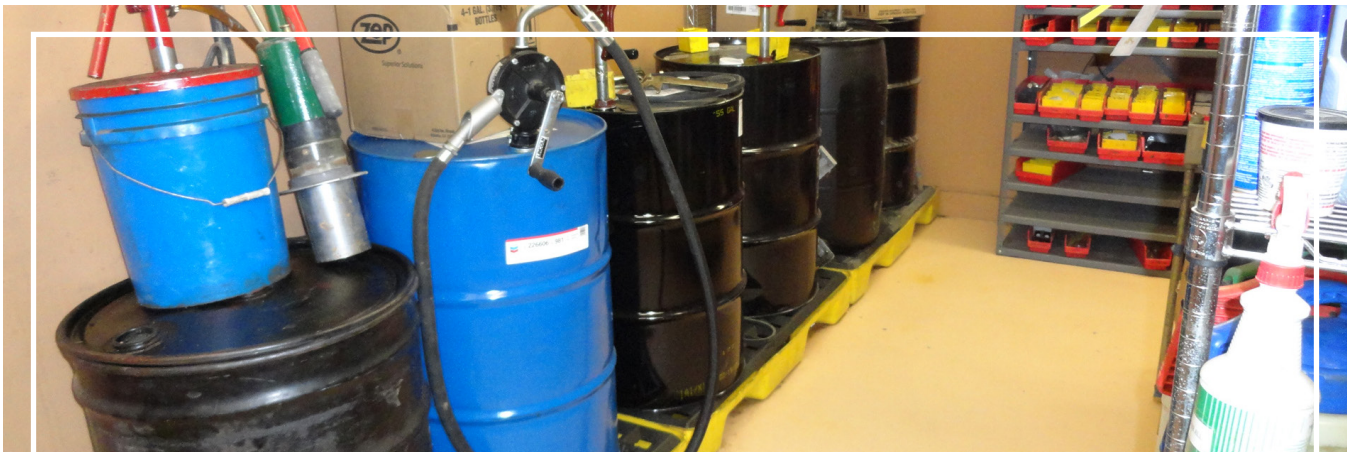
Commercially available products such as these under the drums can provide effective containment.
